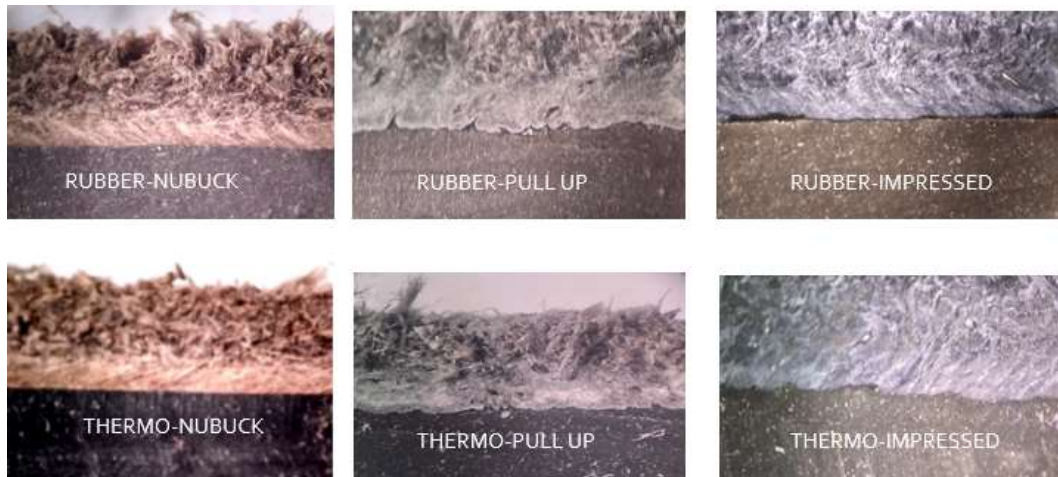
Fig.5. Optical microscope images of sticked samples
